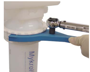
4 Tighten locking ring to easily seat double O-rings. Use a torque wrench to ensure proper tightening.
